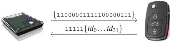
Figure 10: Message flow for reading memory block 0
