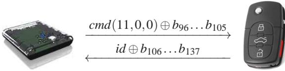
Figure 13: Read *id* without redundancy messages
