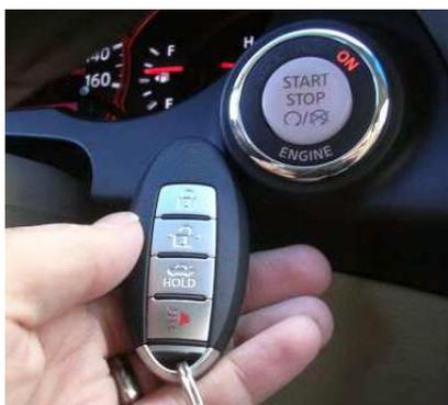
Figure 3: Keyless hybrid transponder and engine start/stop button
