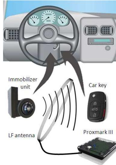
Figure 5: Experimental setup for eavesdropping
