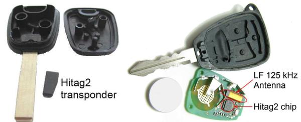
Figure 1: Car keys with a Hitag2 transponder/chip
