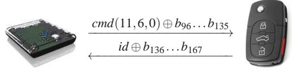
Figure 14: Read *id* using 6 redundancy messages
